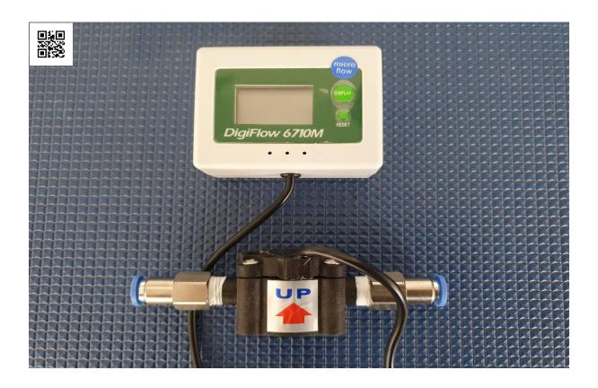
Digital flow meter for De-Bubbler 265 calibration, with programmable volume and time periods. Measures flow rate and total volume of water. Suitable for use with water. 0.05~1.0 litres per minute, 8mm OD fittings.
